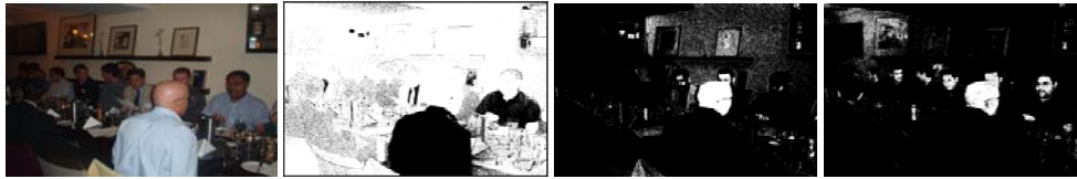
Fig 4. Skin detection in an arbitrary image: (left to right) original input image (image 8 in Table 1), skin tone detected by [4], by [25] and by the proposed method in this work respectively.
