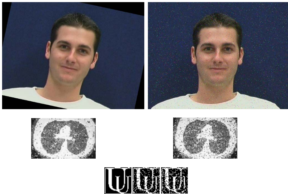
Fig 12. Resistance to image processing attacks: (left) attacked stego-image with a joint attack of cropping and rotation of -12 degrees and the extracted secret data, the little error in the extracted signal is due to interpolation operation (right) attacked with salt and pepper noise and the extracted secret data, (bottom, left to right) successful extraction of embedded data after JPEG compression with quality factors Q=100 , Q=80 and Q=75 respectively.
